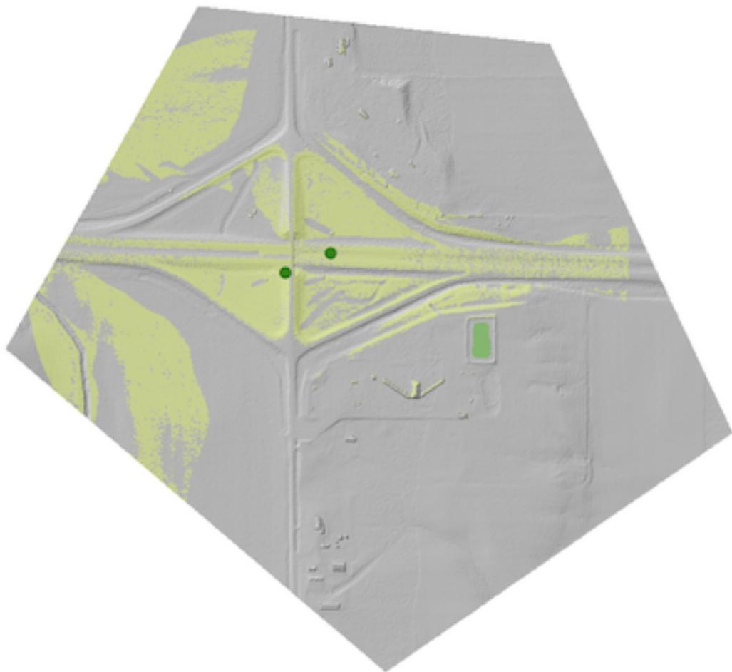
Fig. 1: A computed visibility for two separate -ox and -oy points on a DEM.
