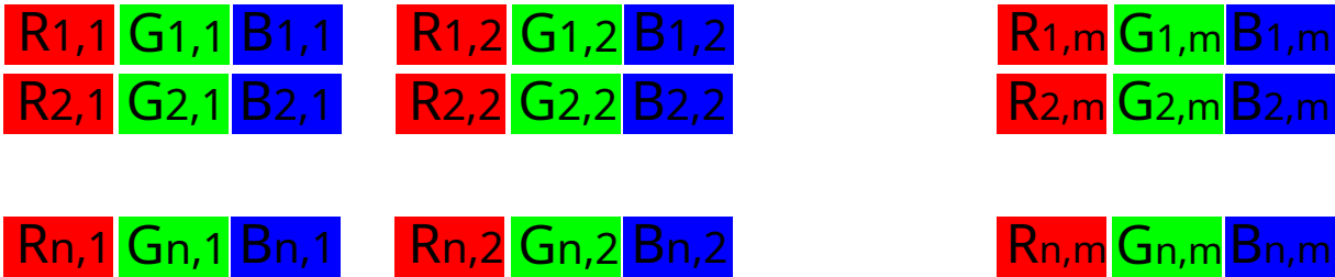
Fig. 1: Band Interleaved by Pixel (BIP) mode
